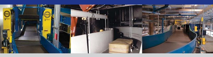
Vertical sort units are used in-line with the security scanning conveyor belts to remove suspect baggage to off-line baggage inspection. Laser scanners read bag tag barcodes to determine the destination flight and assigned make-up location in order to activate in-line bag sorters. Transportation conveyors quickly deliver bags from the screening room to the make-up room.
