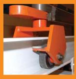
Friction Drive Wheel – comes in contact with load bar to move carrier –
