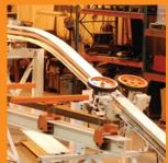
**Track Switch** – allows friction conveyor to operate like power & free
